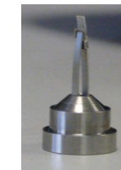
Figure 8. A section of chip mounted in a modified cryopin. Each section of chip contains up to 4 chambers. Each chamber typically contains between 1 and 20 crystals, enabling the simultaneous mounting of ~4-80 crystals per pin.
