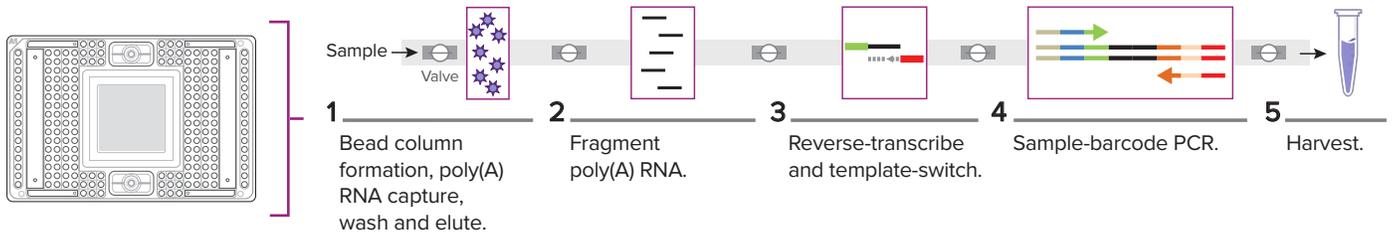
Figure 2. The 48.Atlas IFC architecture automates multiple workflow steps otherwise performed manually, including poly(A) RNA capture, RNA fragmentation, reverse-transcription, sample-barcode PCR and multiple wash steps.
