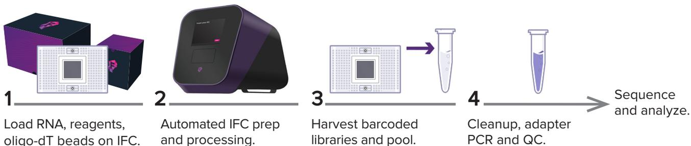
**Figure 1. Advanta RNA-Seq NGS Library Prep Kit workflow on Juno.** Samples and Advanta RNA-Seq reagents are added to the 48.Atlas IFC, which is subsequently processed on the Juno instrument. The system solution automates many tedious hands-on steps to generate up to 48 RNA-seq libraries. The nanoscale design of the 48.Atlas IFC significantly reduces reagent consumption, which helps minimize overall costs per sample.
